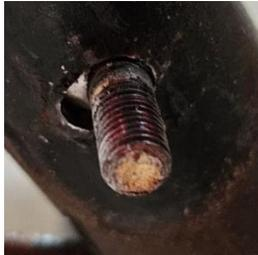
The right leg was still 'intact' but also showed elongated holes. The bolt was also impacted and was collapsing.
