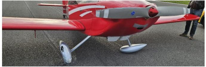
Investigation revealed that a bolt in the left wheel strut was broken and the hole was bulged out due to extreme shimmy.
